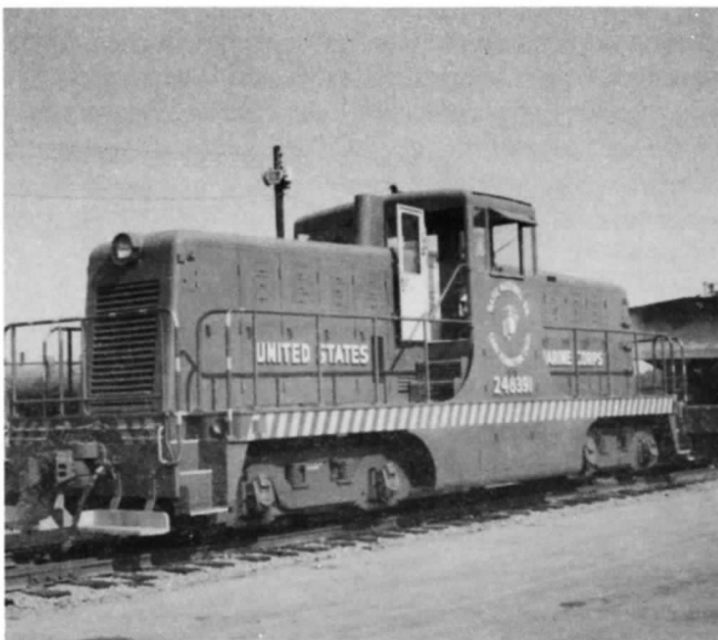
No. 24831, G.E. 80 tonner of 1944, is still serving the Marine Base.
