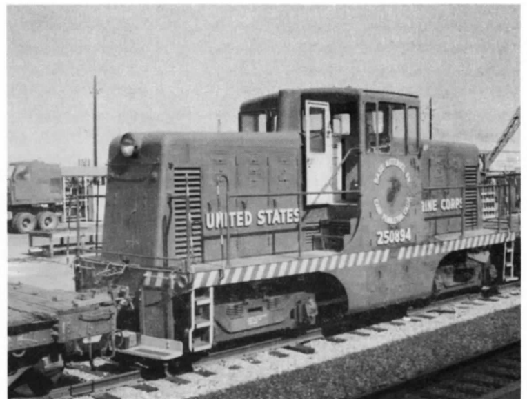
Built in 1942, this 44 ton unit now works the Naval Station in San Diego.
