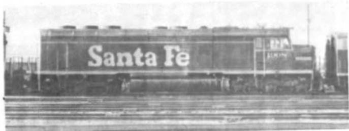
EMD / F45 / 3600 hp / 6 axles C-C wheel arrangement SANTA FE 5900-5939 (1900-1939)
